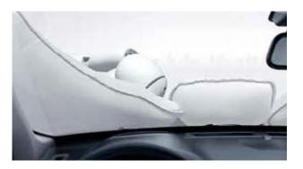
DRIVER VISIBILITY The airbag deployment has been designed to ensure that the effect on the driver's vision is minimised.
