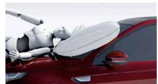
ENHANCED PROTECTION The shape of the deployed airbag offers enhanced protection to a pedestrian in the event of an impact.
