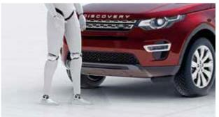
PRESSURE SENSORS The system uses advanced pressure-tube sensors, located in the bumper, to detect impact.
