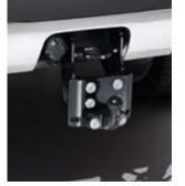
Multi-height tow hitch allows for three different tow-ball height positions. Simple to fit, once armature installed, and can be swapped between positions in seconds. 50mm tow ball is included and will take up to 3,500kg trailer load and 350kg nose weight. Requires tow eye cover.
