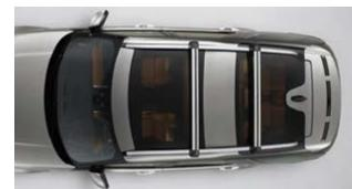
Roof Rails\* VPLRR0156 – Silver VPLRR0155 – Black (not shown) Roof rails facilitate easy fitment of cross bars for roof carrying. Pre-set positioning points ensure cross bars are fixed in optimum position for weight distribution and dynamics. Maximum payload 80kg.\*\*
