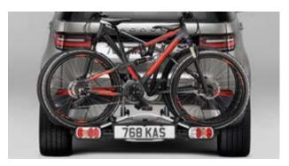
Tow Bar Mounted Bike Carrier VPLVR0067 – 2 Bike Carrier<sup>†</sup> VPLVR0069 – 3 Bike Carrier<sup>†</sup> (not shown) Tow bar mounted bike carrier available for two or three bikes. A quick
