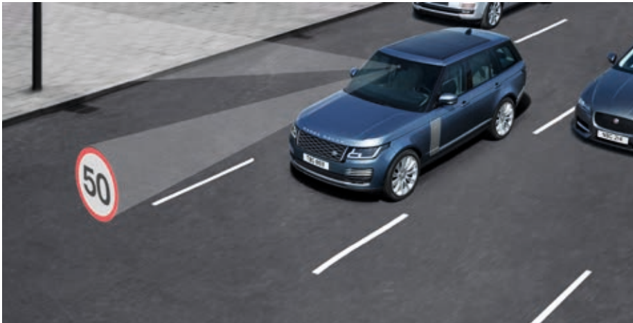
Traffic Sign Recognition with Adaptive Speed Limiter
