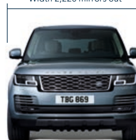
Width 2,073mm mirrors folded Width 2,220mm mirrors out
